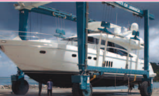
Yachts up to 100 ft in length and 100 tonnes can be handled
