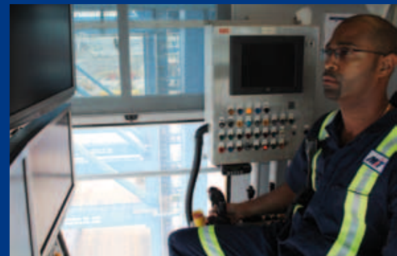
The fixed cabin created a more comfortable work environment, with crane operators able to perform in a more natural, upright position.
